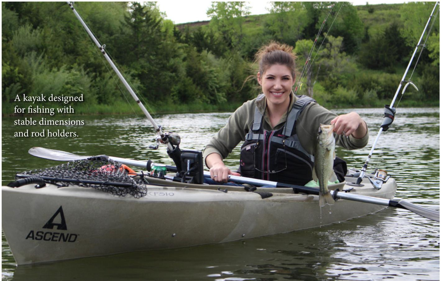
A kayak designed for fishing with stable dimensions and rod holders.
